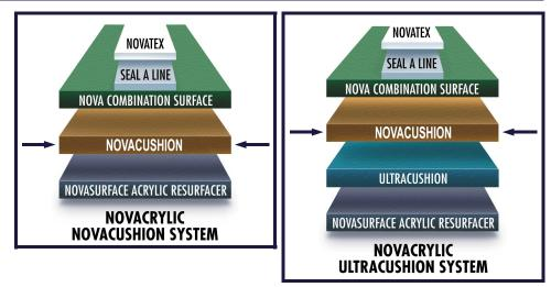
After the application of NOVACUSHION is completed, 2 coats of COMBINATION SURFACE should be applied. This results in a uniform texture and appearance.
